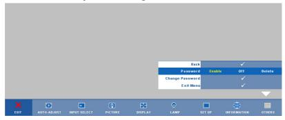
**b** Enabling the Password function will pop up a character screen, key in a 4-digit number from the screen and press .
